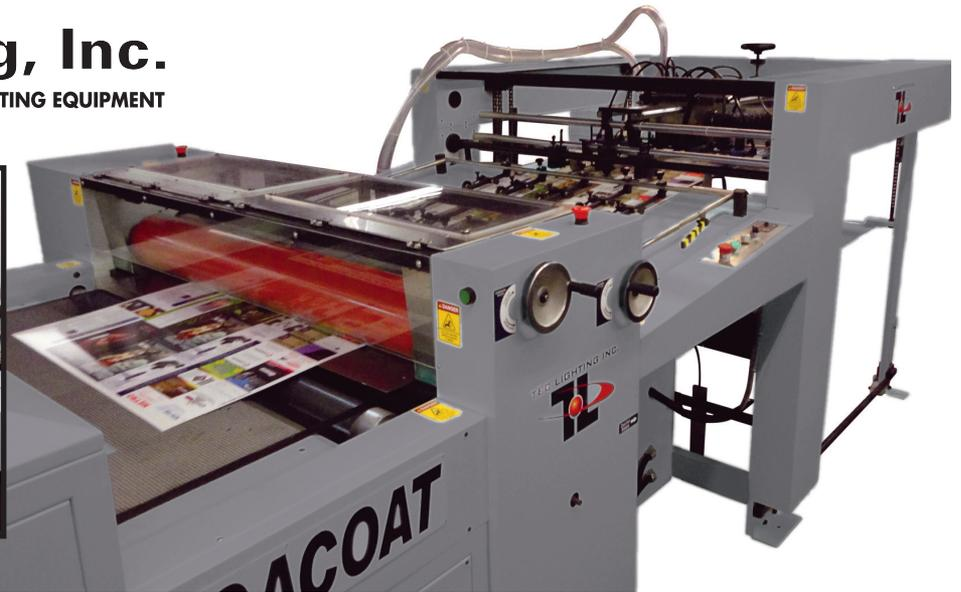
The MegaCoat UV Coater is a high production UV coater designed for the most demanding workload of mid/large offset printers looking to add flood UV coating offline. This machine is a cost effective alternative to the high cost of adding a UV coating station on press.
