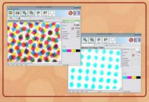
Image Color Separation & Analysis from printed halftones, separated and analyzed for true halftone dot area analysis & correction. Useful for printing without targets.
