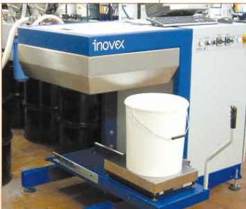
Scale slide assists in manual additions & removal of pail
